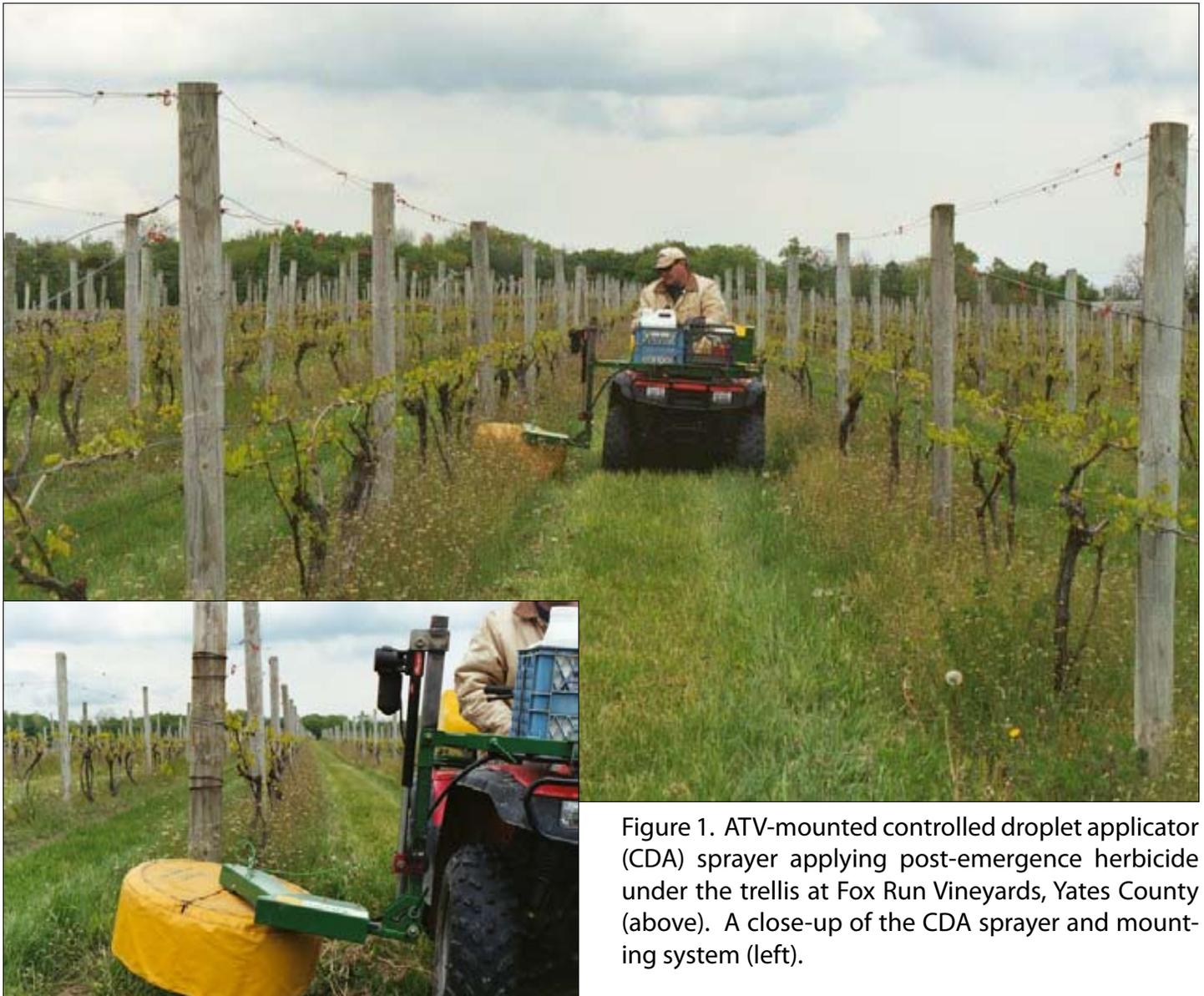
Figure 1. ATV-mounted controlled droplet applicator (CDA) sprayer applying post-emergence herbicide under the trellis at Fox Run Vineyards, Yates County (above). A close-up of the CDA sprayer and mounting system (left).
